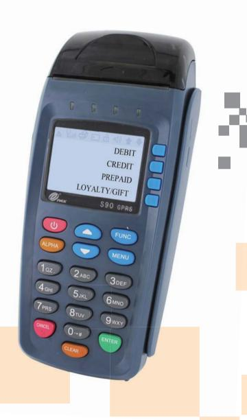
PAX's S90 mobile POS terminal has been designed to offer superior wireless performance, embedded in a ruggedized yet stylish form factor. With options for single SIM or dual SIM functionality, and with a large memory and a high capacity Li-ion rechargeable battery, the S90 is one of the most popular mobile terminals with merchants today.
